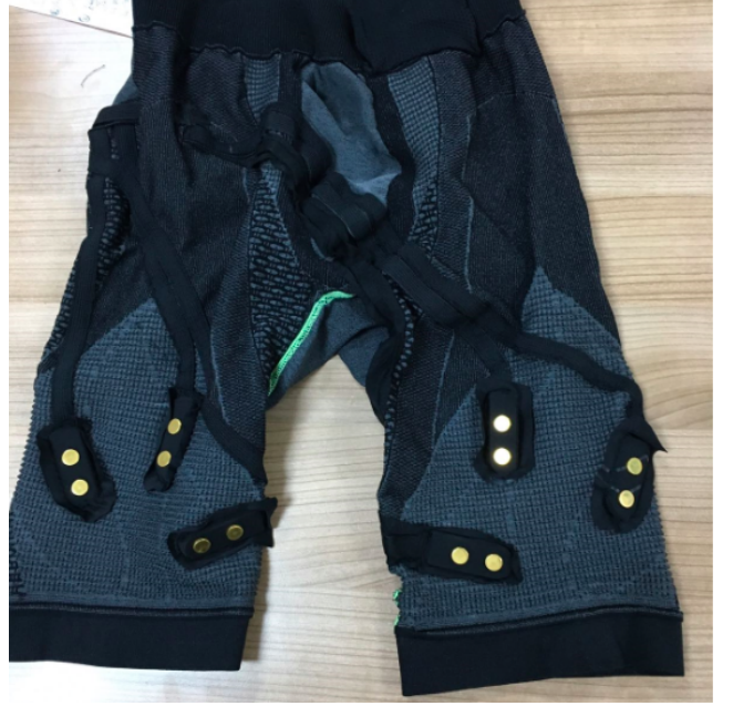
Figure 1: Visual of the sEMG Data Acquisition System.
